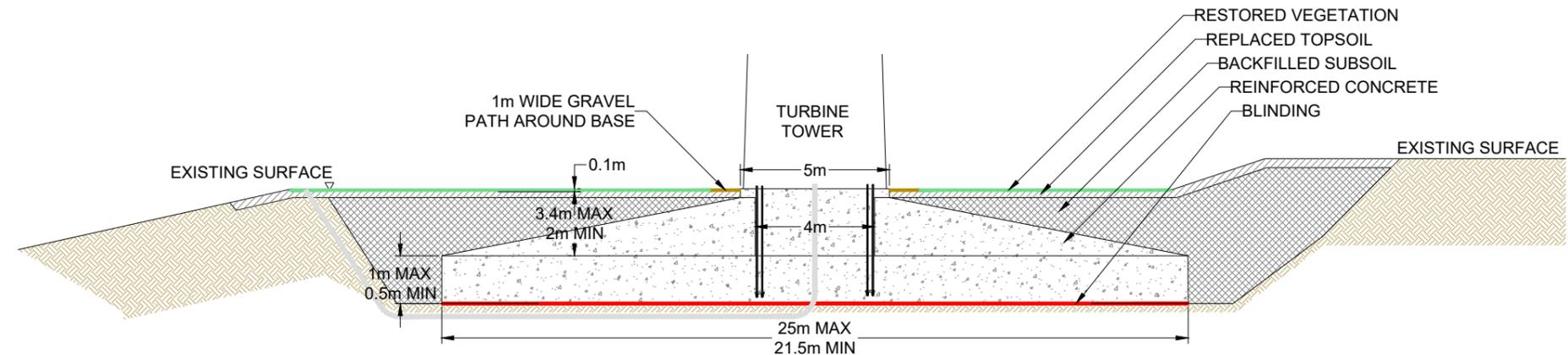
**TYPICAL TURBINE FOUNDATION SECTION**
